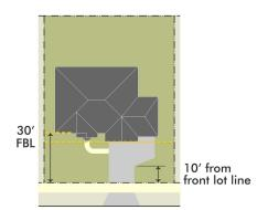
Figure 5-7 Application of Driveway Limits
