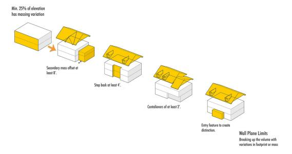
Figure 5-10 Wall Plane Limits
