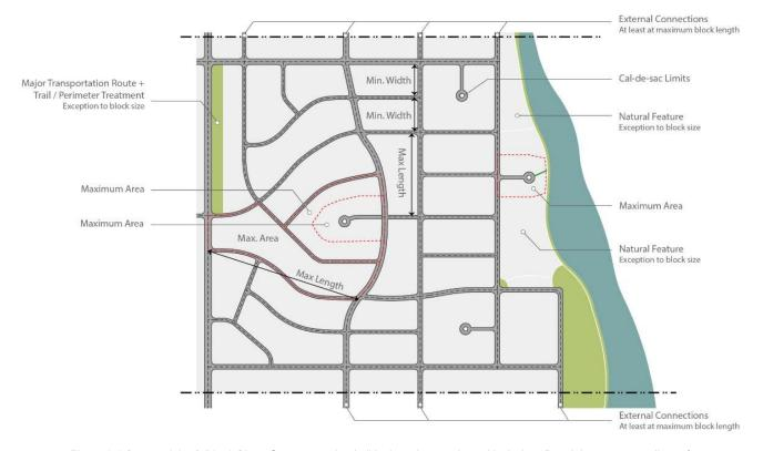
Figure 3-1 Connectivity & Block Sizes. Street networks shall be based on maximum block sizes (length between centerlines of perimeter streets and area) and stub to adjacent property at a frequency sufficient to create connected networks unless exceptions justify not connecting.
